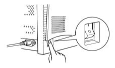
The Control Panel displays a blinking "1" and the machine starts to warm up. The machine is ready to read data when the "1" stops blinking.
